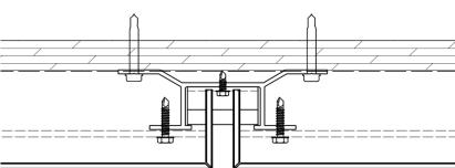
THE SERIES 72 is a hook and pin style system with no caulk or silicone and virtually maintenance free. This panel system features a continuous vertical channel with adjustable panel support pins. The panel returns are notched to hook over the support pins. This completed system is very clean and attractive.
