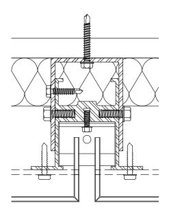
THE SERIES 72 is a hook and pin style system with no caulk or silicone and virtually maintenance free. This panel system features a continuous vertical channel with adjustable panel support pins. The panel returns are notched to hook over the support pins. This completed system is very clean and attractive.
