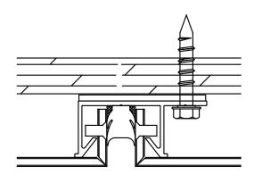
THE SERIES 42 is easy to intall due to the semi-continuous attachment extrusions and the innovative lock-in-place backer wedge. This system is available as a silicone gasket. Since the Series 42 is a non-progressive system, any panel can be removed or replaced without removing adjacent panels, further adding to the desirability of this system. The Series 42 allows for thermal movement and when installed, it offers and holds clean lines and optimizes panel to panel alignment.
