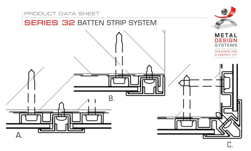
Series 32 is a batten strip system where there are three extrusion types (pictured above), and each type has three pieces. The extrusion types are A: Joint, B: Perimeter, and C: Outside Corner. the pieces are base, retainer, and cover. The non-progressive install is very easy with flat ACM pieces sliding into the extrusions. This all aluminum batten system is an innovative interior or exterior option.
